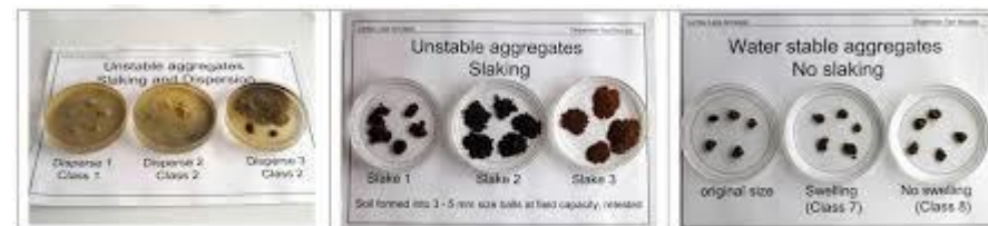
Figure 1. Assessment of appearance of air-dry peds in artificial effluent (SAR 5; EC 1 dS/m).
