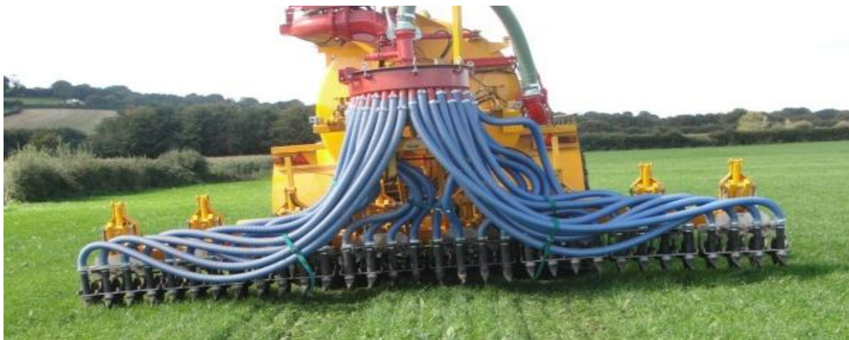
Trailing shoe spreading digestate at Langage Farm, Higher Challonsleigh, near Plymouth
