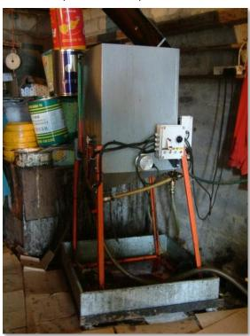
Waste vegetable oil is collected from fish and chip shops and wholesalers and used to make the bio-diesel in a small purpose-built reactor (see below).
