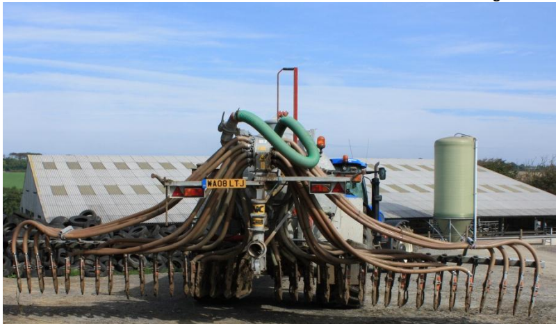
Left: The trailing shoe Right: The slurry being applied to the soils surface
